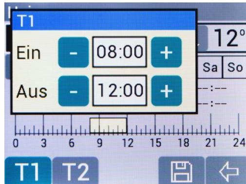
Now set the desired switch-on or switch-off time with the **+** and **-** buttons. The minimum interval length is  $\frac{1}{2}$ h.
