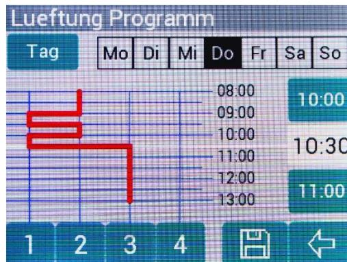
In this screen, the ventilation programmes can be adjusted according to your needs.
